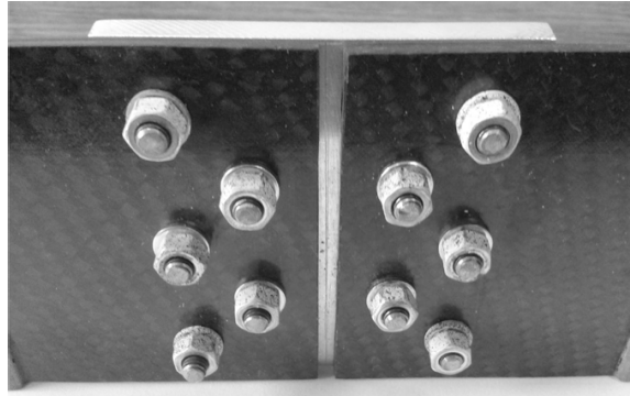
Fig. 5. General view of a composite specimen with two-row bolted joint.
