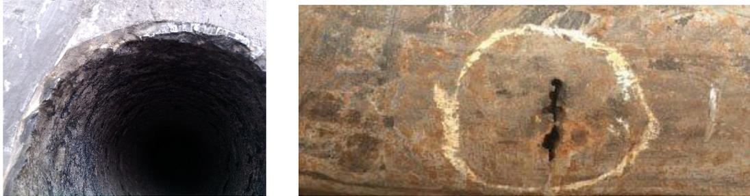
Fig. 1 Corrosion damages of drill pipes
